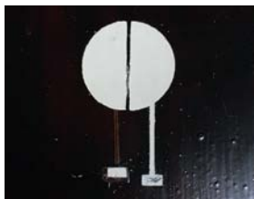
Figure 13: Urushi circuit without coating the urushi layer.
