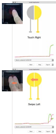
Figure 9: Test application detecting a touch on the right part (top) and left swipe (bottom).
